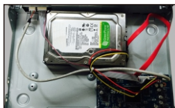
④ Connect the power and data cables.
