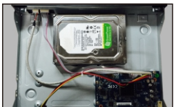
③ Place the HDD onto the bottom of the case.
